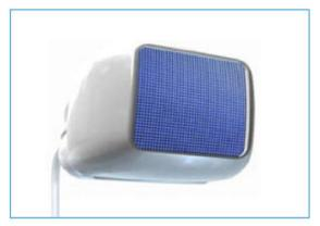
xMATRIX array technology utilizes 2400 fully-sampled elements for 360-degree focusing and steering.
