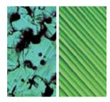
Conventional PZT ceramics (as shown to the left) are made up of randomly oriented grains, while PureWave crystals (shown at the right), have a virtually perfect atomic level arrangement and uniform consistency throughout the material.
