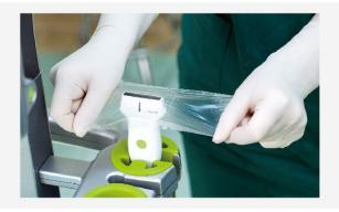
Recognize the probe direction mark (probe mark is corresponding to red round icon on screen).
